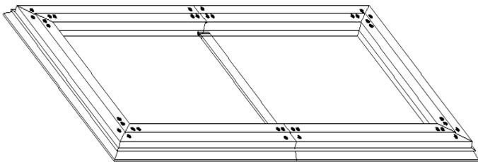
2. Remove self-adhesive backing and Adhere LED Strip all around the rear side edge of Frame as pictured.
