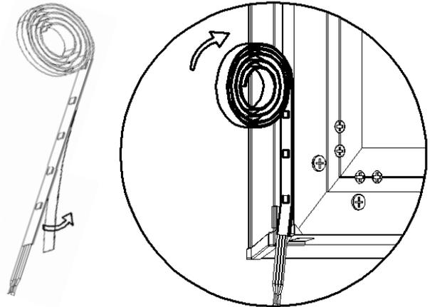
3. When adhering LED Strips, adhere one strip around the frame one direction and the second strip in the other.
