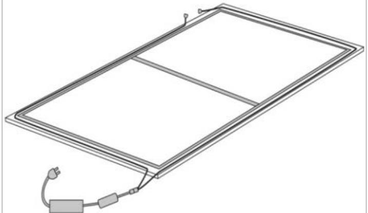
\*After the LED strip has been applied along the entire rear edge of the frame, if there is excess to the LED backlighting strip, you are able to remove any excess backlighting strip by simply cutting the strip along the indicated line. See following images shown:
