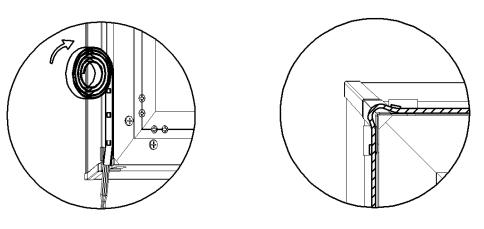
Step3. Secure the LED light strip by using the LED clips as shown below.
