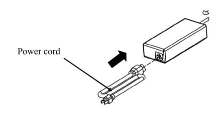
**Step 5.** Connect the LED Controller to the Power Supply
