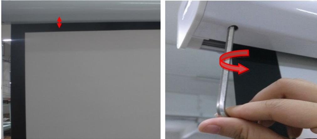
To decrease the drop of the screen: Press the down button on the remote to lower the screen. Insert the Allen wrench into the lower limit adjustment screw and turn the limit screw clockwise. (1 full turn equals about 1")
